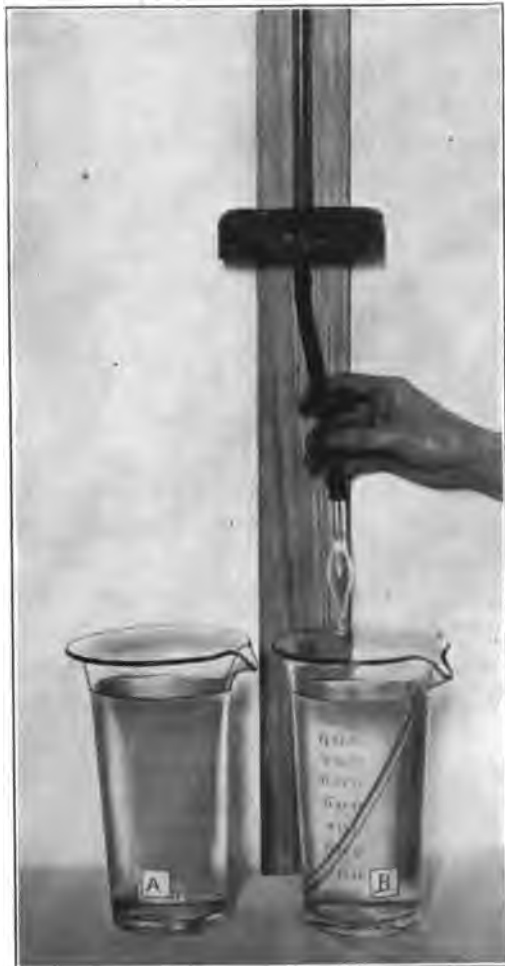
FIG. 157.—APPARATUS TO DETERMINE AMOUNT OF INDIGO-CARMIN IN THE URINE. Apparatus consists of two beakers of 1,000 c. c. capacity each, a burette graduated in hundredths of a c. c., and a pipette graduated in hundredths of a c. c.
